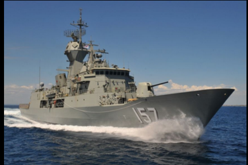
HMAS Perth with a Phased Array Radar from CEA Technologies in Canberra
